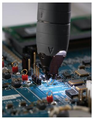
Figure 2. N2750A Series differential probe with browser tip
